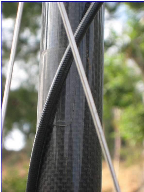
Sette Frame Patch Protectors to protect the carbon's clear coat finish from the dreaded brake hose
