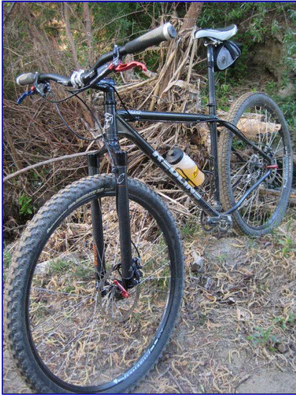
Full bike setup: fully rigid, with 2.35 inch tire Panaracer Rampage up front
